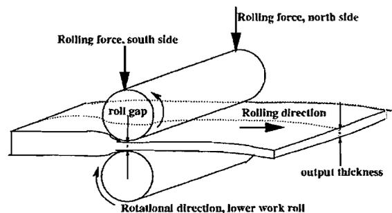
Figure 1: The rolling process, side view. The plate moves from left to right, and the upper roll moves up and down. The gage between rolls defines the output thickness of the plate.
