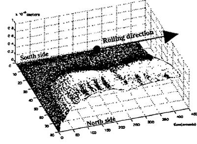
Figure 4: Representation 3D of the space-state computed thickness error
