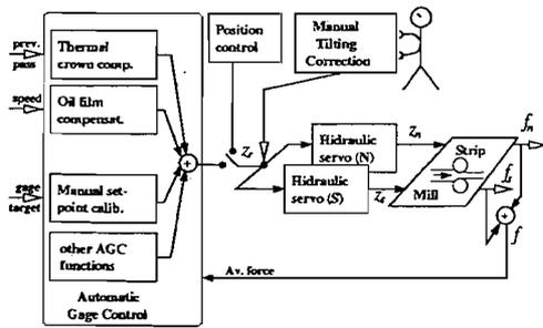
Figure 2: Building blocks of an AGC. The human operator controls the unevenness position of the rolling cylinders
