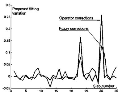
Figure 5: Comparative of the correction *tilting* signals proposed by the human operator and the fuzzy controller for a set of 33 rolling passes.
