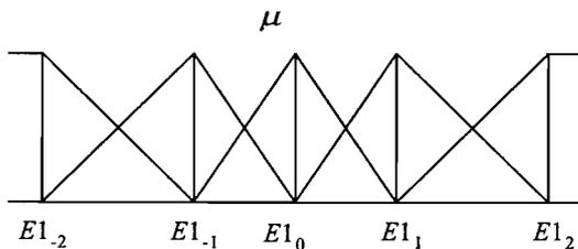
Fig. 1 Unequally spaced membership function.
