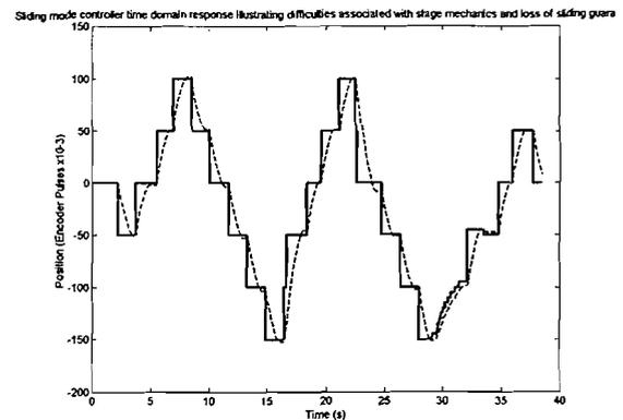
Figure 5: Real time sliding mode controller response
