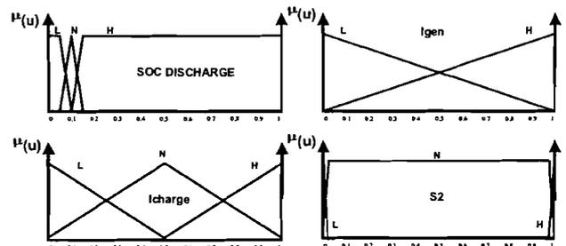
Figure 6: Fuzzy Set for overdischarge control system.
