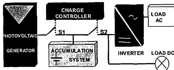
Figure. 1: Stand-alone Photovoltaic System.
