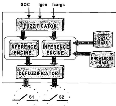
Figure 4: Structure of Fuzzy Charge Controller.
